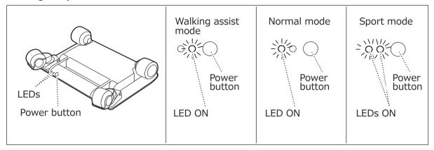
Press the power button to turn the power ON.
