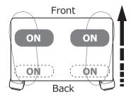
Speed increases when 2 sensors on the front are turned ON.
